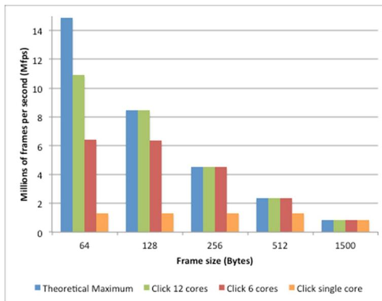
Figure 9. Raw frame throughput with different frame sizes.
