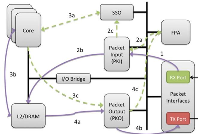
Figure 4. Simplified OCTEON packet flow [4].
