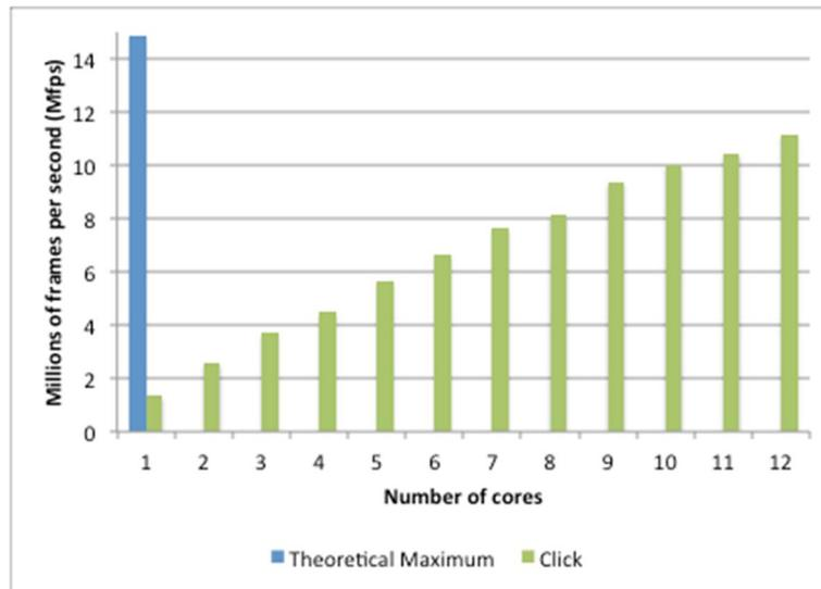
Figure 7. Raw frame forwarding rate with minimum sized (64 Bytes) Ethernet frames.
