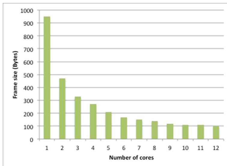
Figure 8. The minimum frame size to reach line speed.
